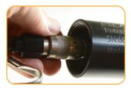
If your Pro-X has a Twist-Lock cable, slide it onto the instrument and twist until it clicks into place.
