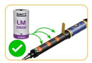
For best battery life, install Li-MnO<sub>2</sub> batteries purchased from In-Situ. Alkaline batteries are intended only for simple, short-term deployments at moderate temperatures.
