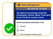
By default, VuLink is set to power connected instruments with every reading. Go to **Power Manamgement** and change this setting to **Never** if the instrument has its own power. Some instruments or complex networks require more power and may result in shorter battery life. These include:
