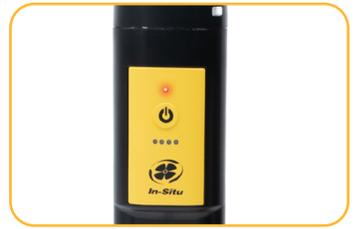
Press the power button and check that the Connection Status LED is solid.
