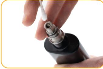
Clean dirty connector pins with alcohol. Do not allow water to get into connector.
