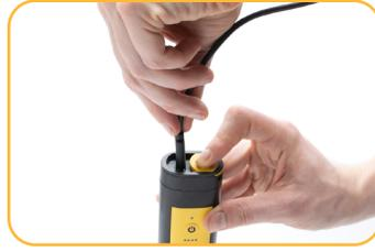
Use the USB-C cable to charge the device.
