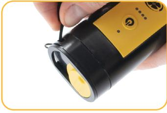
Thread the loop through the slot on the TROLL Com Plus.
