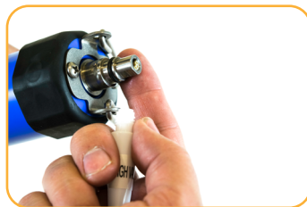
Ensure O-ring on instrument connector is clean. Apply vacuum grease to O-ring.
