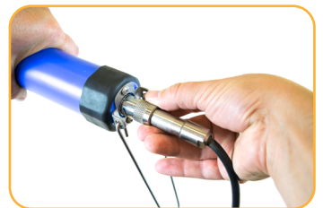
Hold textured sleeve of cable in one hand and instrument in other. Push and twist until click.
