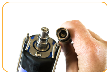
Flat edge inside cable end must align with flat edge on instrument connector.
