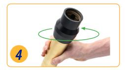
Gently shake the sonde in a circular motion to rinse the inside of restrictor and sensors.
