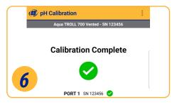
Pour calibration solution into the restrictor 1 cm above the sensors and cover with the end cap. Follow the instructions in VuSitu to start the calibration.
