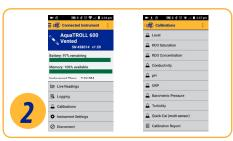
In VuSitu, click **Calibrations** from the Connected Instrument screen and choose a sensor to calibrate.
