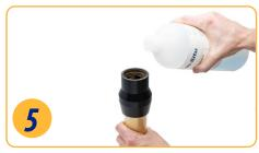
Discard the DI water and repeat rinsing procedure two more times with 10-20 mL of your first calibration standard.
