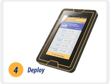
Perform a 100% saturation calibration to adjust for changes in altitude or barometric pressure. Connect to VuSitu and choose Calibrations. Then follow the on-screen instructions to complete the calibration.
