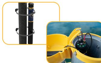
Secure VuLink and instruments in the final deployment location.
