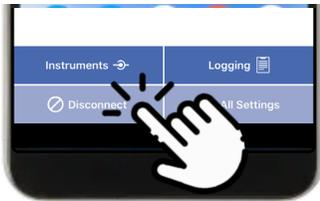
Before inserting the SIM card, disconnect VuLink from VuSitu.
