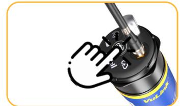
Press the button on the VuLink to initialize the SIM card.
