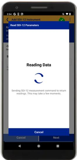
VuLink will send a Measurement command (aM!) and Send Data (aDO!...) commands to the instrument.
