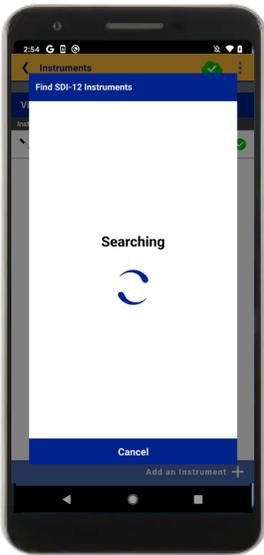
VuLink will send an Identification command (a!) to the instrument.
