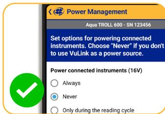
By default, VuLink is set to power connected instruments with every reading. Go to **Power Management** and change this setting to **Never** if the instrument has its own power. Some instruments or complex networks require more power and may result in shorter battery life. These include:
