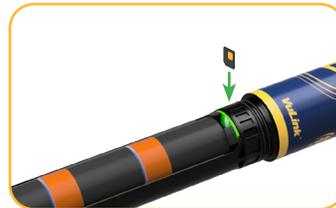
Insert the SIM card into the SIM compartment inside the battery cover.
