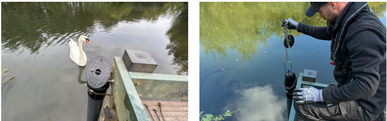
Figure 2: Stilling tube (left) and sonde deployment (right) at the monitoring site.
