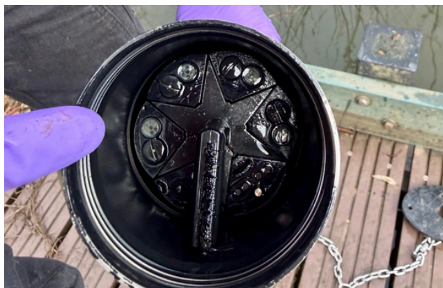
Figure 3. Sensors deployed on the In-Situ Aqua TROLL 800 multiparameter sonde: four ammonium sensors, pH, and conductivity/temperature.
