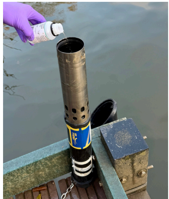
Figure 5. (a) The 1 mg/L ammonium standard solution (top) and (b) the sonde with restrictor reversed to use the mini-calibration cup for the weekly standard measurement (bottom).
