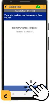
If you are using VuLink, add the instrument. Then tap the instrument to connect.
