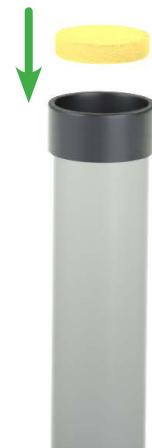
Saturate the sponge wafer (use approximately 10 mL of water) and place it in the bottom of the calibration chamber.
