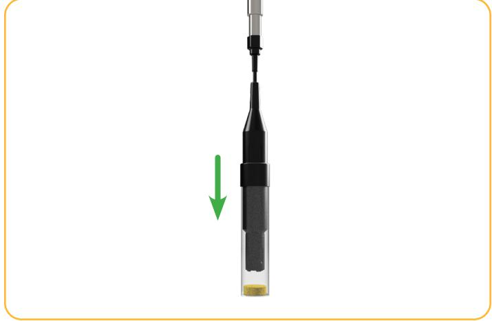
Place the probe in the calibration chamber so that the sensing element is about 2.5 cm (1 inch) above the water-saturated sponge.
