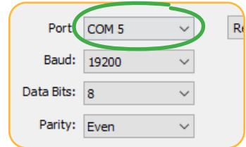
If the software does not connect to the software, you can find the COM port your computer has assigned in Windows Device Manager > Ports.
