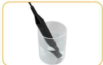
To remove extensive mineral build-up, soak the probe cap-down in vinegar for 15 minutes. Then soak in deionized water for 15 minutes.
