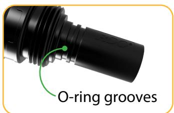
Use your finger to apply a light layer of silicone-based lubricant around the O-ring grooves.
