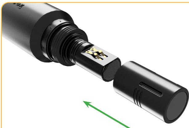
Align the RDO cap so the flat edge on the inside matches up with the flat edge on the sensor. Slide the RDO cap into place.
