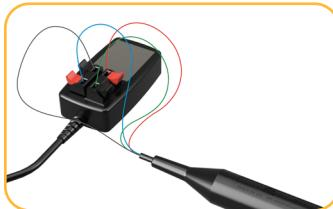
To attach the sensor to the communication device, depress a lever and insert the appropriate wire in the location specified by the diagram.
