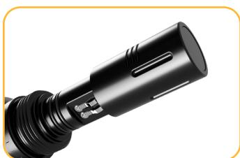
Align the flat edge inside the RDO cap with the flat edge and metal contacts on the probe. Slide the cap in place.
