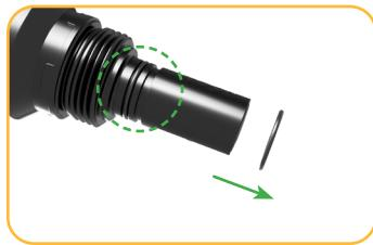
Remove the existing O-rings from the sensor.
