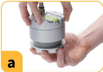
Remove the nut from the base of the Level TROLL NC.
