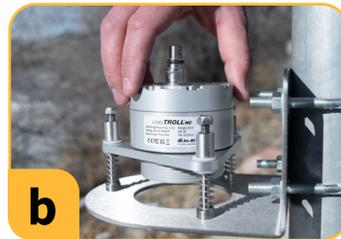
Thread Level TROLL NC into instrument holder. You may need to disconnect longer cables to complete this.
