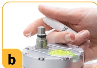
**b** Apply a small drop of grease to the O-ring if it is dry.
