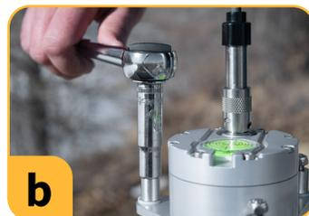
Use a socket wrench with a 10 mm deep socket to adjust the leveling bolts.
