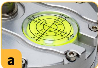
Use the bubble level on the top of the instrument to view sensor tilt.
