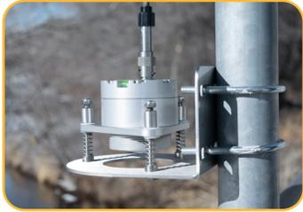
Strap mounting bracket to vertical pole with U-bolts.
