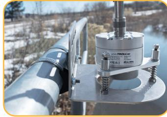
Strap mounting bracket to horizontal railing.
