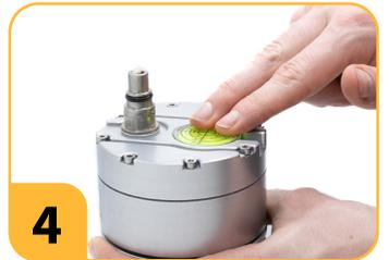
**4** Press down on the new level to secure it in place on the instrument.
