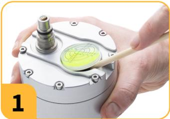
**1** Use a plastic or wooden tool to gently remove the bubble level.
