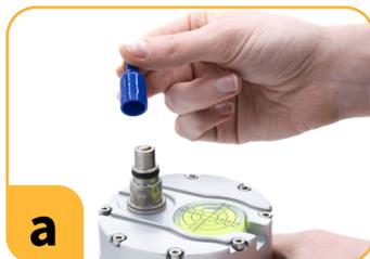
**a** Remove protective caps from instrument and cable.
