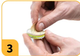
**3** Peel the paper from the back of the new level to expose the adhesive.
