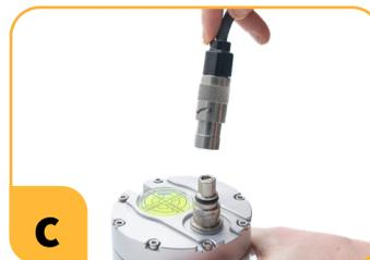
**c** Align flat edges of cable and connector.
