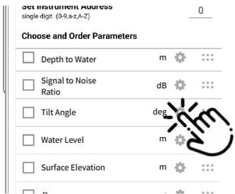
Tap the gear icon to adjust the units for each parameter.
