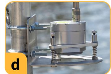
Optional: Reinstall the nut onto the instrument base for added security.
