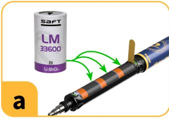
If you are using VuLink, install Li-MnO<sub>2</sub> batteries.
