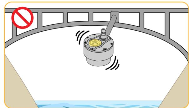
Significant vibration can cause readings to fluctuate.
